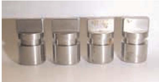
TWO-HOUR salt spray test per ASTM B-117 (With passivation on the left and without on the right.)
