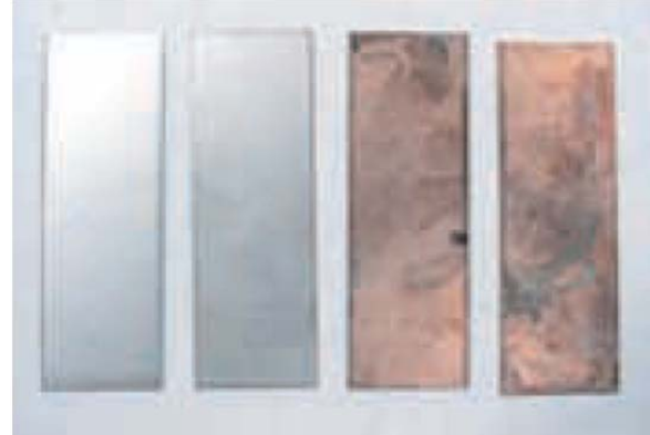
Copper Sulfate test per MIL-STD-753. (With passivation on left and without on right.)
